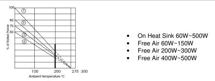
Fig - Maximum dissipation (Pmax) in percentage of rated power as a function of the ambient temperature (Tamb)
