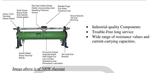
Rheostats are mainly used for regulating electric current in industry and laboratory where these are used as adjustable resistors in electrical circuits. With three terminal provisions, these can also be used to vary a D.C. potential smoothly from zero to maximum.
